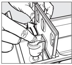
Over time, detergent residue can build up in the water jets in the top of the detergent drawer housing.
